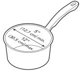
should have a flat, heavy magnetic bottom and straight sides with a diameter of 5" (13 cm) to 12" (31 cm) to accommodate the various sized elements. The induction cookware should be in good condition and free from excessive dents on the bottom to provide maximum performance and convenience.
